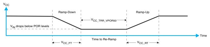
Figure 26.  $V_{CC}$  is Lowered Below the POR Threshold, Then Ramped Back Up to  $V_{CC}$
