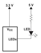
Figure 22. Device Supplied by a Lower Voltage
