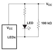
Figure 21. High-Value Resistor in Parallel With LED
