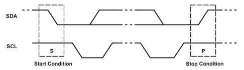
Figure 15. Definition of Start and Stop Conditions
