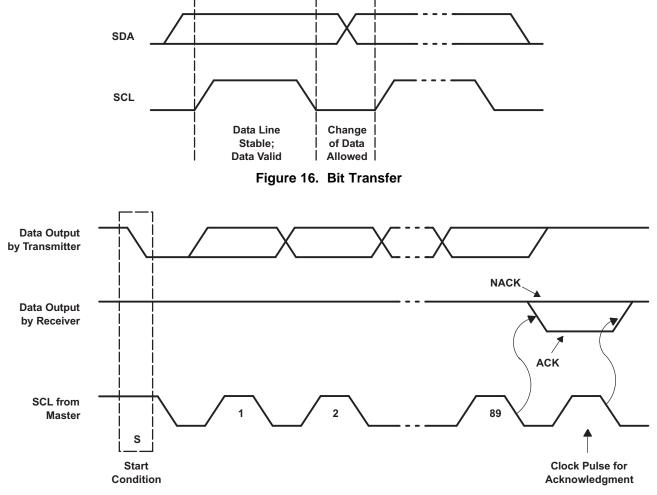
Figure 17. Acknowledgment on I<sup>2</sup>C Bus
