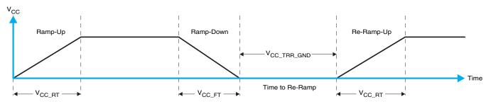
Figure 25.  $V_{CC}$  is Lowered Below 0.2 V or 0 V and Then Ramped Up to  $V_{CC}$
