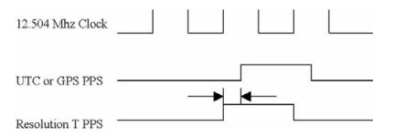
The amount of quantization error present on each PPS output pulse is reported in packet 0x8F-AC. This quantization error information can be used to reduce the effective amount of jitter on the PPS pulse.
