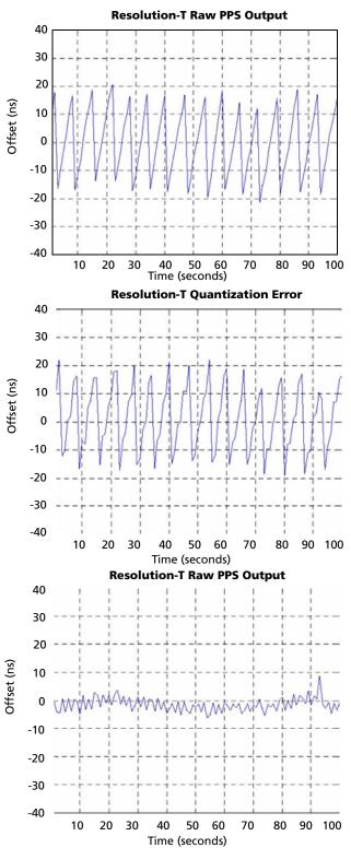
quantization error as reported by the Resolution T in packet 0x8FAC. The bottom plot is the result of subtracting the quantization error from the PPS offset.
