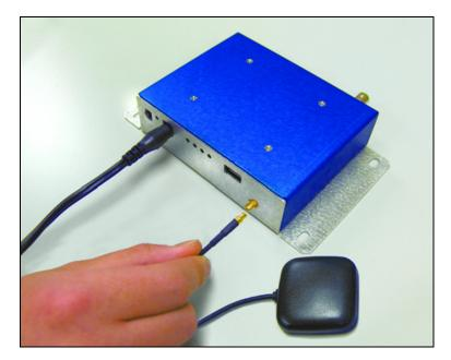
9. Connect the magnetic mount GPS antenna to the interface unit:
